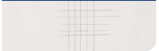
Aged Alkyd Adhesion - Unsanded Substrate (Dulux 23010)
